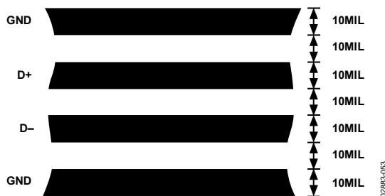
Figure 54. Arrangement of Signal Tracks
